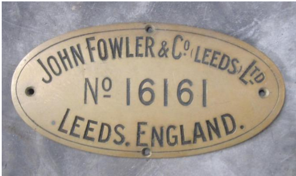
The manufacturer's plate, showing the engine's number, attached to the side of the boiler above the belly tank. The separate boiler number is too obscured by wear to photograph effectively.
